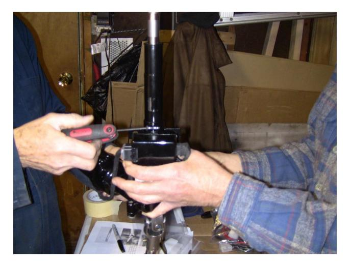
The original snap off bolts had an insert that protected the lock cap. Use caution when drilling out the bolts on a drill press not to damage the insert. (These were Not supplied by EZ.) You can see the locking bar here that fits into the slot of the steering shaft.
