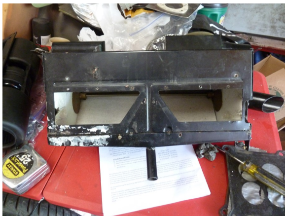
Heater Box showing the openings for the fan.
